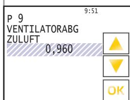
**P 9 Ventilatorabgleich Zuluft**
